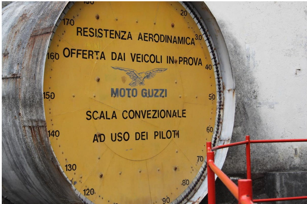
Photo 2. Real time display of drag for rider information
