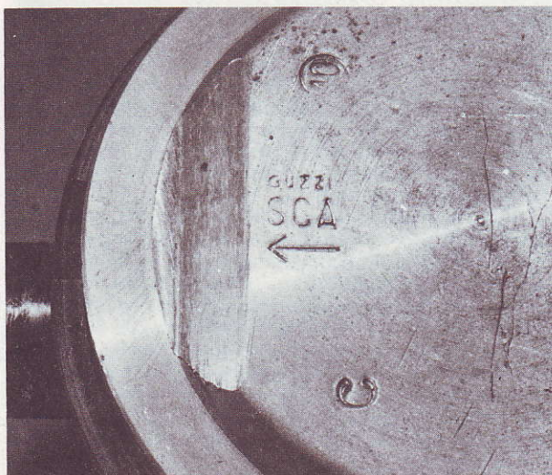
19.2 Mark 'C' on piston indicates cylinder/piston classification
