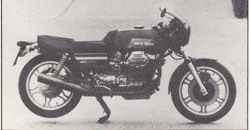
Progressive wound springs at the back provide sophisticated damping. Shrouded dampers inside the springs keep out the muck and bullets; it's a firm ride at the back end but my no means too stiff. Likewise the front. The forks travelled well, and never bottomed. They rode bumps like a valkyrie on heat. In common with other shaft-drive machines, the shaft and its housing are utilised as one swing-arm.
