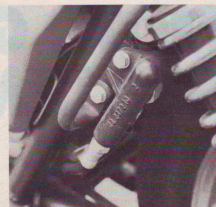
Proportioning valve distributes braking force from rear master cylinder: 70% to rear brake, 30% to front.
