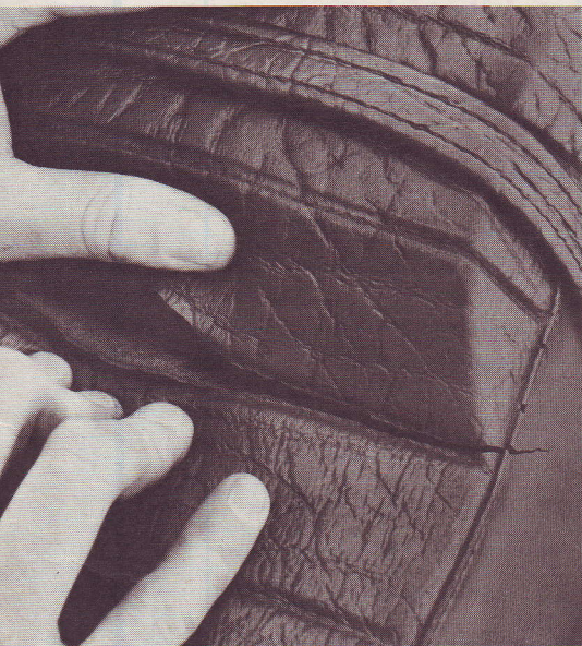
The seat developed a tear at the base of the passenger kick-up; this was not unique to just this bike.
