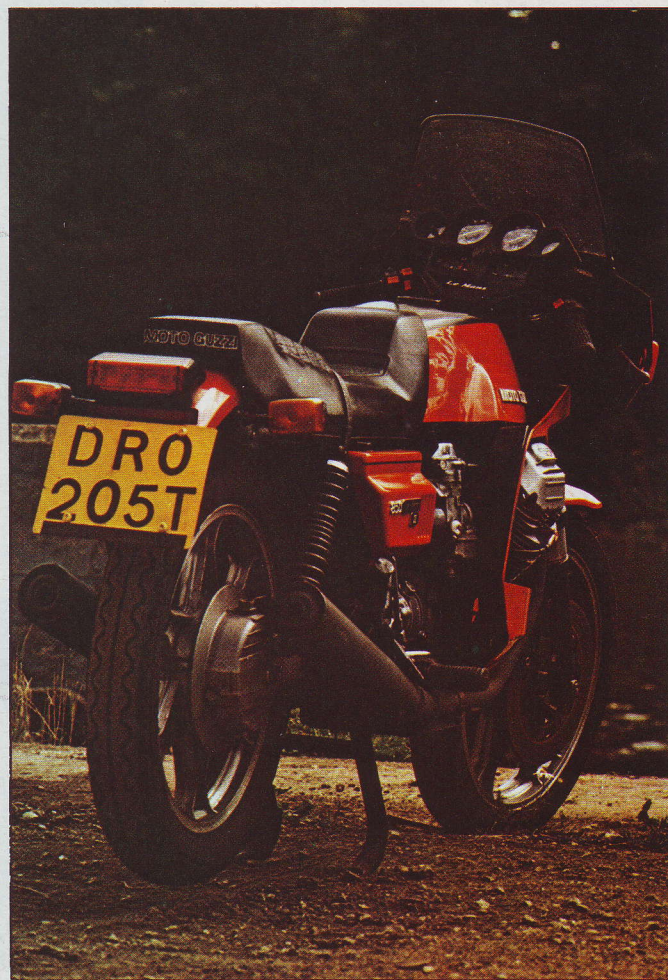
Left: The design of the fairing allows good cooling for the pots and some warm air through to the legs. Above: Black exhaust and rear shock springs contribute to the Guzzi's understated look.
