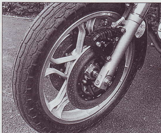
Twin discs sit up front. Brakes are Brembo, naturally, and front and back are linked.
