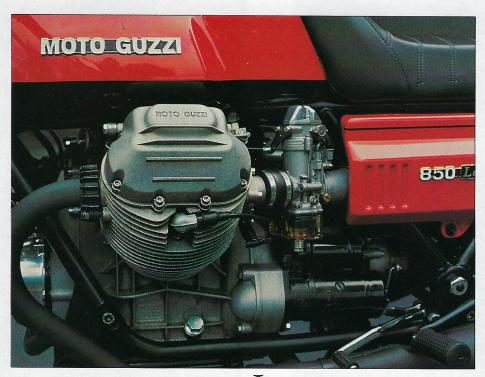
Above: All engine and transmission seals were replaced during Guy's Guzzi restoration, as was about 99% of all existing hardware.
