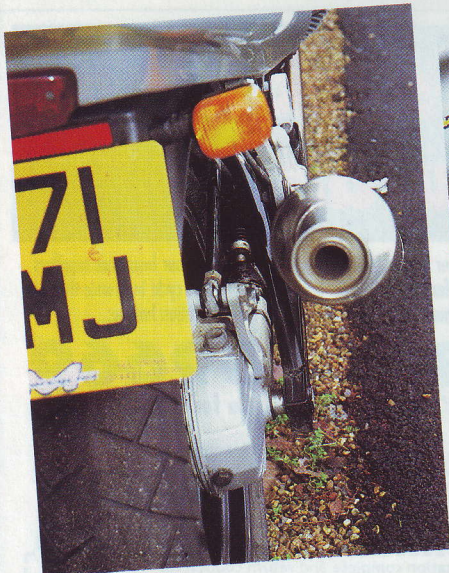
Sport's suspension is more or less separate to the drive system. Torque reaction is lost in the frame/engine
