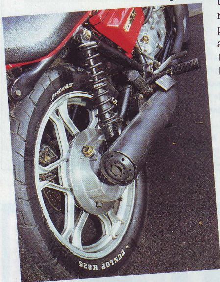
Lemon's suspension function is hampered by the fact that one end of one shock is attached to the drive box
