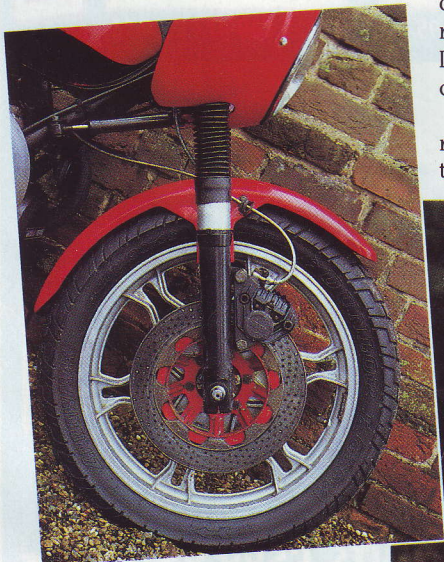
Brakes on both bikes are Brembo; the Lemon's were traditionally praised for power, but slagged for feel ('wooden' was the cliché). The Sport's are beyond criticism
