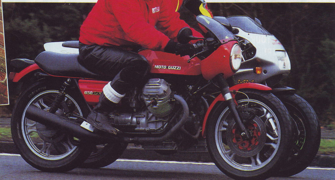
Brakes on both bikes are Brembo; the Lemon's were traditionally praised for power, but slagged for feel ('wooden' was the cliché). The Sport's are beyond criticism
