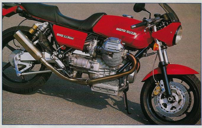
Main: **Engine** is angled down at the back as can be seen in this picture **Bottom Left** Steering damper is highest quality Ohlins unit **Bottom Right** Large Dell Ortos pump the juice for the near half litre cylinders
