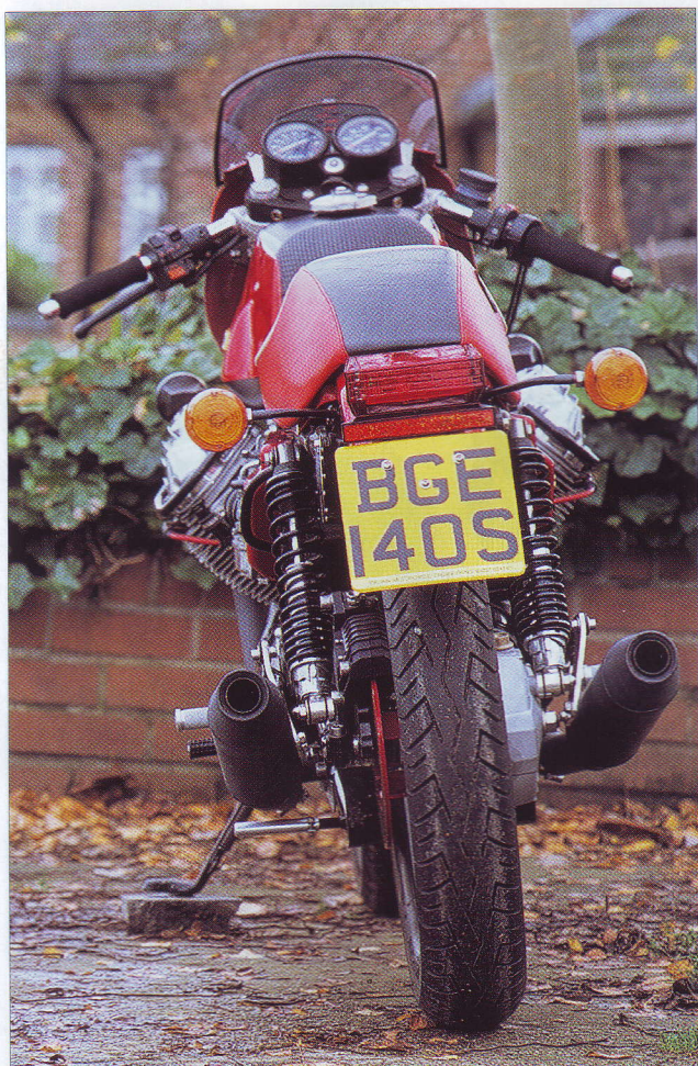
From this view – with down-turned bars, fly screen, twin pipes and those protruding cylinders – it could only be a sporting Guzzi.
