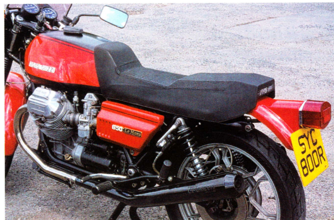
Seat is a moulded rubber item – this one, from a Mk II model, provides slightly more room for a passenger than the original.
