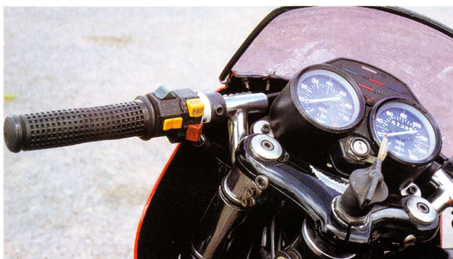
Switchgear for the lights, horn, turn indicators and dip beam all in one neat unit. Friction steering damper supplements a hydraulic damper mounted below the tank.
