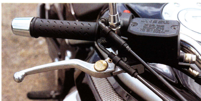
Griso handlebar levers feature span adjusters – if only Moto Guzzi had used these 30 years ago!
