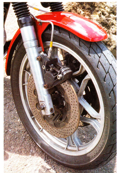
Brembo disc brakes established a benchmark that has seldom been met by others, even today.
