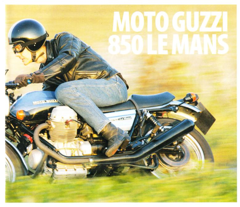
just over 130mph. That was serious speed when the Le Mans was introduced in 1976. Guzzi's work in uprating the 750 S3 model's engine with 844cc capacity, increased compression ratio, bigger carbs and a new exhaust system had resulted in an 80bhp maximum that was matched by only a handful of rivals.
